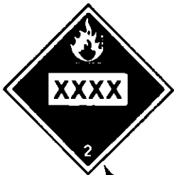
NUMBER 2 FLAMMABLE GAS
