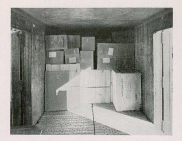
When the entire transloaded lot consists of cartons and boxes the load is levelled off and stowed solid. When package freight must be loaded with rough freight, bulkheads are installed. Note letters "L.A." indicating destination of complete shipment on top box and "L" on each box in this car.
