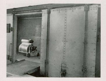
A Silent Glow Car Dryer removes all traces of moisture from refrigerator cars, which makes them perfectly dry for shipping merchandise cargo whether the contents be packed in a cardboard carton, a sack container, or similar type material. Special heaters can also be placed in refrigerator cars when merchandise is perishable, such as, drugs, candies, etc., and needs heat protection during extremely cold weather while in transit.
