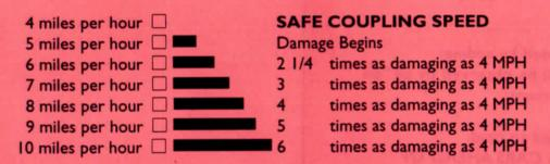
Damage to freight or car can be avoided by always keeping coupling speed within the safe range.
