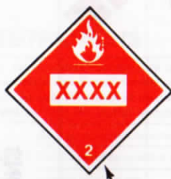
NUMBER 2 FLAMMABLE GAS
