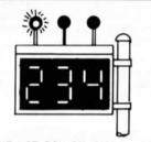
ONE HOT BOX ON RIGHT SIDE OF TRAIN IN DIRECTION OF MOVEMENT. AXLE COUNT (234) FROM REAR OF TRAIN. INSPECT ALL BEARINGS OF CAR INDICATED AS WELL AS EACH ADJOINING CAR.
