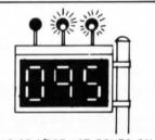
TWO OR MORE HOT BOXES ON LEFT SIDE OF TRAIN IN DIRECTION OF MOVEMENT. AXLE COUNT (095) FROM REAR OF TRAIN, INSPECT ALL JOURNALS, REAR OF TRAIN TO AND INCLUDING CAR AHEAD OF AXLE COUNT ON DISPLAY.
