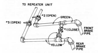
Note: If for any reason it becomes necessary to transfer control of air brakes to the helper engine located in the portion of the train behind the RAC car with the RAC air equipment in operation, the brake pipe hose connections must be changed. The forward brake pipe must be coupled to the portion of the train having the brake valve which is controlling the train. The rear brake pipe must be coupled to the other end of the train.
