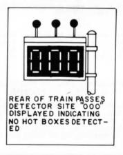
The indicator lights are normally dark, but when hot bearing is detected, will display flashing white aspect as illustrated below:
