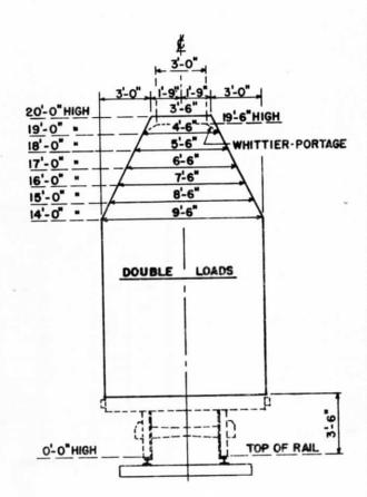
Maximum Loading Diagram For Single And Double Loads
