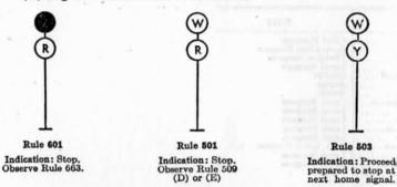
Aspects displayed by westward MAIN TRACK leaving signal located near M. P. 320.9 (Snake Lead).
