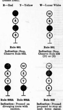
Aspects displayed by westward YARD leaving signal located between tracks No. 1 and 3 near M. P. 320.9 (Snake Lead).
