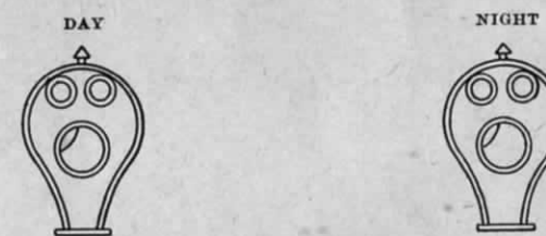
Distant Disc Signal. Indication: "Proceed."
