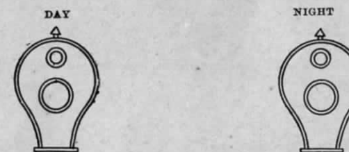
Home Disc Signal. Indication: "Stop."
