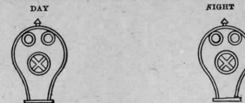
Distant Disc Signal. Indication: "Proceed with caution to Home Station."
