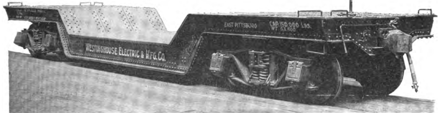
Car of 250,000 lbs. Capacity for Shipping Transformers.
