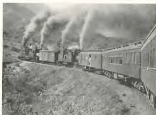
Passenger Train Hauled by Two Double-ended Steam Locomotives up 4½-per cent Grade North of LaBota
