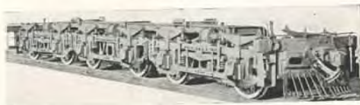
Running Gear of 150-ton Articulated Type Locomotive
