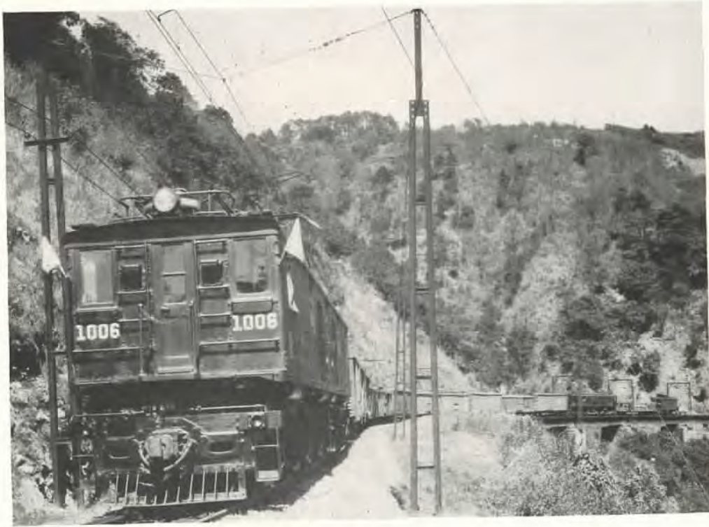
Mexican Railway Company Freight Train Hauled by Two 150-ton Electric Locomotives
