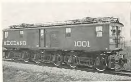
One of the 150-ton, 3000-volt Direct-current Locomotives
