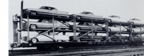
LO-DEK 89 and TRI-LEVEL AUTO RACKS —The LO-DEK 89 accepts all makes and models of tri-level auto racks. The increased deck length allows application of new design auto racks with greater length and overhead clearance and permits the hauling of 12 standard or 15 compact autos.
