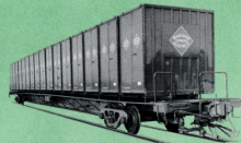
P-S MODULAR CONTAINER CAR. The Pullman-Standard Modular Container Car is a new concept of container carrying rail equipment. Essentially a center sill riding on two sets of trucks, the car will accommodate sixteen 8'x8'x5' Trailmobile containers or any mix of containers up to 80 feet in length. The Pullman-Standard Container Car can be equipped for passenger train operation and meets all ICC and AAR requirements for a car of this type
