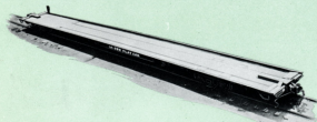
P-S LO-DEK FLAT CAR. The lowest flat car on the market (only 31 inches from rail to deck) the LO-DEK is now also the longest: 89 feet. This added length means added versatility for the growing piggyback movement and provides increased room for the cushioning of both trailers and containers. High strength steel construction, all-steel deck and combination rub rails and side sills mean extra economy . . . reduced maintenance.
