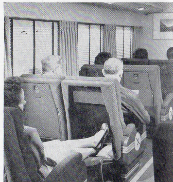
A leg rest adds to the travel ease of coach passengers on the Empire Builder, new Great Northern streamlined train.—Great Northern Railway.
