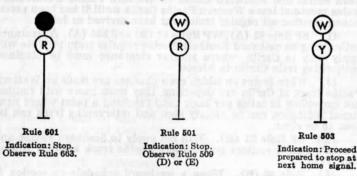
Aspects displayed by westward MAIN TRACK leaving signal located near M. P. 320.9 (Snake Lead).
