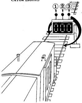
The diagram depicts a Type C hot box detector's monitor display board and indicator lights as it would be viewed looking back after rear of train has passed detector site. The indicator lights indentified ①②③ are normally dark, but when a hot bearing is detected, lights ① (right side) or ⑤ (left side) will immediately display a flashing white light to identify the side of train on which the hot bearing was detected.
