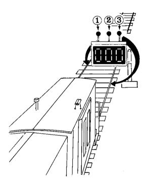
The diagram depicts a Type C hot box detector's monitor display board and indicator lights as it would be viewed looking back after rear of train has passed detector site. The indicator lights identified OOD are normally dark, but when a hot bearing is detected, lights O (right side) or O (left side) will immediately display a flashing white light to identify the side of train on which the hot bearing was detected.
