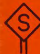
STATION ONE MILE SIGN. ONE MILE FROM FIRST SWITCH OF SIDING ON SINGLE TRACK IN TRAIN CATER TERRITORY. NOT USED ON BRANCH LINES
