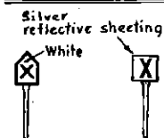
HIGHWAY GRADE CROSSING WHISTLE SIGN
