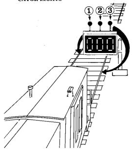
The diagram depicts a Type C hot box detector's monitor display board and indicator lights as it would be viewed looking back after rear of train has passed detector site. The indicator lights indentified ©30 are normally dark, but when a hot bearing is detected, lights © (right side of train) or ③ (left side of train) will immediately display a flashing white light to identify the side of train on which the hot bearing was detected.
