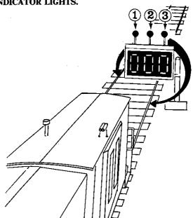
The diagram depicts a Type C hot box detector's monitor display board and indicator lights as it would be viewed looking back after rear of train has passed detector site. The indicator lights identified OOD are normally dark, but when a hot bearing is detected, lights ① (right side) or ③ (left side) will immediately display a flashing white light to identify the side of train on which the hot bearing was detected.
