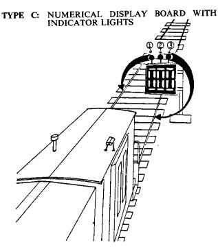
The diagram depicts a Type C hot box detector's monitor display board and indicator lights as it would be viewed looking back after rear of train has passed detector site. The indicator lights indentified O33 are normally dark, but when a hot bearing is detected, lights O (right side of train) or O (left side of train) will immediately display a flashing white light to identify the side of train on which the hot bearing was detected.
