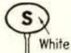
STATION ONE MILE SIGN See Rule 14 (m) (One mile from station or first switch of siding, whichever is nearer, on single track in train order territory. Not to be used on branch lines.)
