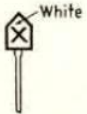
HIGHWAY GRADE CROSSING WHISTLE SIGN 1320 feet from Crossing where speed is 60 mph or less, and 1850 feet where speed is over 60 m. p. h. See Rule 14 (l)
