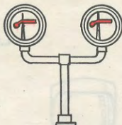
FIG. 2 BLOCK OCCUPIED IN BOTH DIRECTIONS
