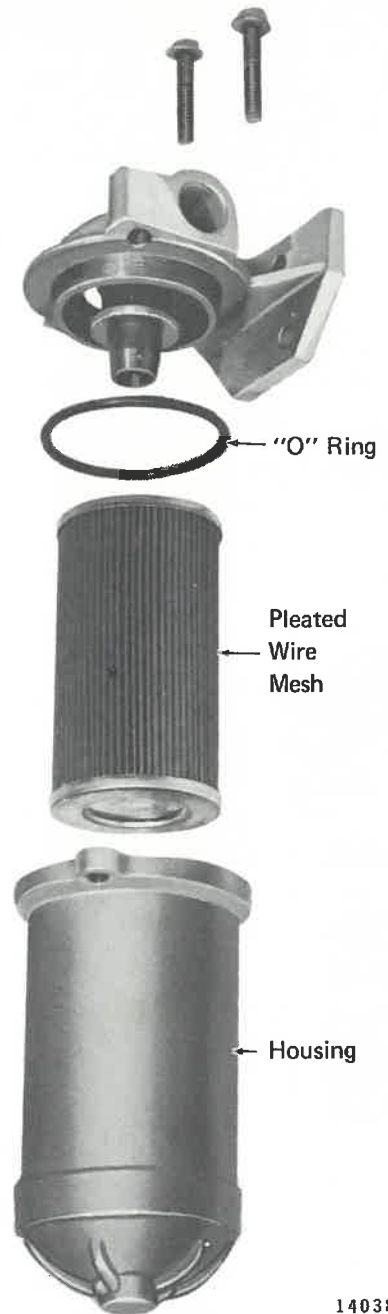
Fig. 1-4 - Fuel Suction Strainer, Exploded View
