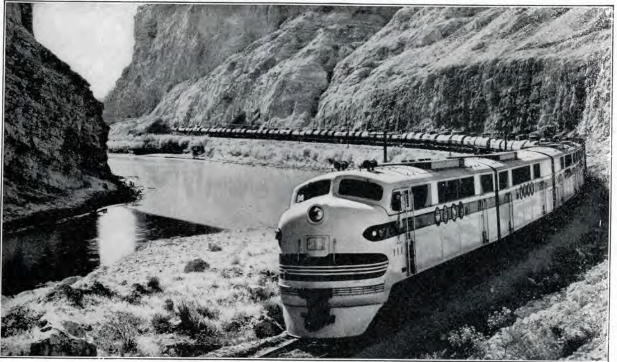
A trainload of oil, pulled by a 4-unit Diesel-electric freight locomotive, speeds through the canyon.
