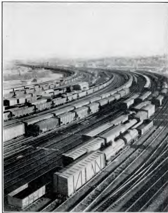
One of hundreds of huge freight classification yards where cars are assembled into trains.
