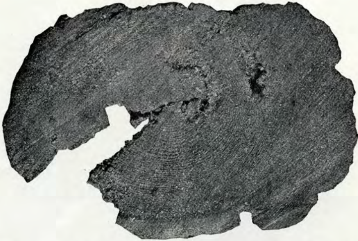
Fig. 1. Section of cedar tie removed from paved streets in Michigan. Tie reported to have been removed in October, 1913, after 8 to 10 years' service. Photo taken in November, 1913.
