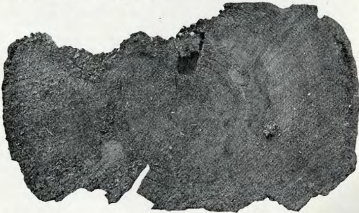
Fig. 2.—Section of cedar tie removed from paved streets in Michigan. Tie reported to have been removed in June, 1913, after 8 to 10 years' service. Photo taken in November, 1913.
