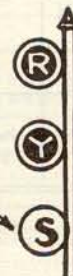
FIG. 180 RULE 290 WITH TAKE SIDING INDICATION BE GOVERNED BY BLOCK SIGNAL INDICATION, OPEN SWITCH & PROCEED INTO SIDING
