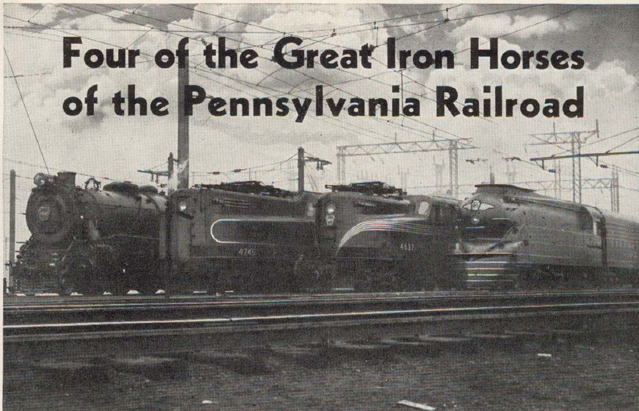
(Left to right) K-4s Standard Pacific Type Locomotive; the P-5A Electric Engine; the new Streamline GG1 Electric Locomotive, and new Streamline Coal-Burning Locomotive . . . . . latest development of Aerodynamic Science
