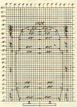
These diagrams show dimensions of maximum load that can be carried over entire system. A load of much larger dimensions can be carried over many portions of the system for which see Standard Clearance Diagrams and information published quarterly in Railway Line Clearances.
