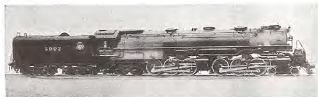
Challenger Type freight locomotives are 100 feet long; capable of pulling a train of 100 loaded cars at mile-a-minute speed; carry 22 tons of coal and 19,000 gallons of water in their tenders. All of this simply means superior freight service for Union Pacific patrons.
