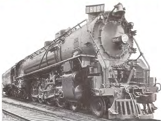
The new high-speed "Challenger" type locomotives have the power to pull 100 loaded freight cars at a mile a minute. Forty of these Union Pacific rail giants are now in use in both freight and passenger service.
