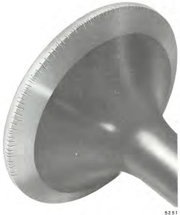
Fig. 2-18 — Face And Rim Defects
