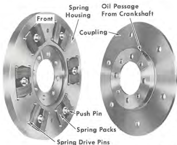
Fig. 5-7 — Harmonic Balancer With Front Coupling Removed
