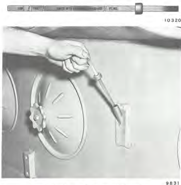
Fig. 8-2 — Oil Level Gauge
