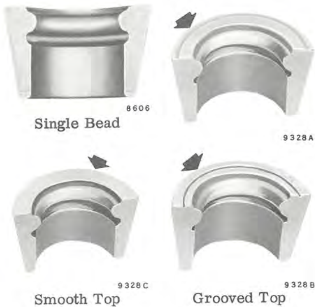
Fig. 2-19 — Valve Spring Seat Locks
