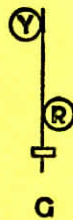
RULE 285 Prepare to Stop at Next Signal. Train exceeding medium speed must at once reduce to that speed.
