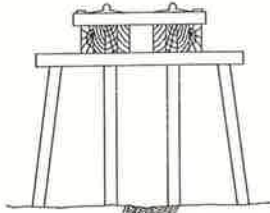
TIMBER PILE TRESTLE-OPEN DECK
