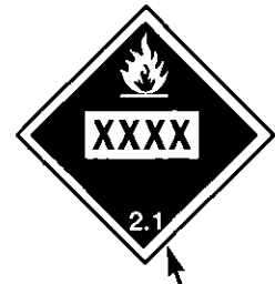
NUMBER 2.1 FLAMMABLE GAS
