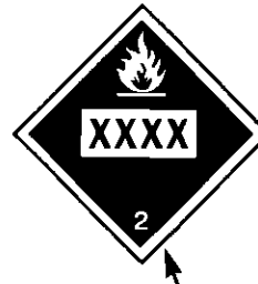
NUMBER 2 FLAMMABLE GAS
