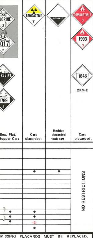
MISSING PLACARDS MUST BE LOCATIONS WHERE CARS ARE INSPECTED SHALL HAVE A SUPPLY FOR THIS PURPOSE. IDENTIFICATION NUMBERS SHALL BE ADDED TO ALTERNATE PLACARDS WITH A BLACK MARKING PEN. CORRECT NUMBERS SHALL BE OBTAINED FROM EXISTING PLACARDS ON CAR OR SHIPPING PAPER
